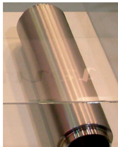
Figure 9: Example of a rotary sputtering target that can be used for a large area Thin Film Technology - Liquid Crystal Display (TFTLCD)
