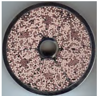
Cross-section of niobium-tin cable, showing central cooling duct (photo: © ITER Organization)
