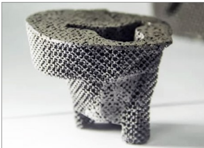
A tantalum knee joint made in 2017 by additive manufacturing (China Global Television Network )
