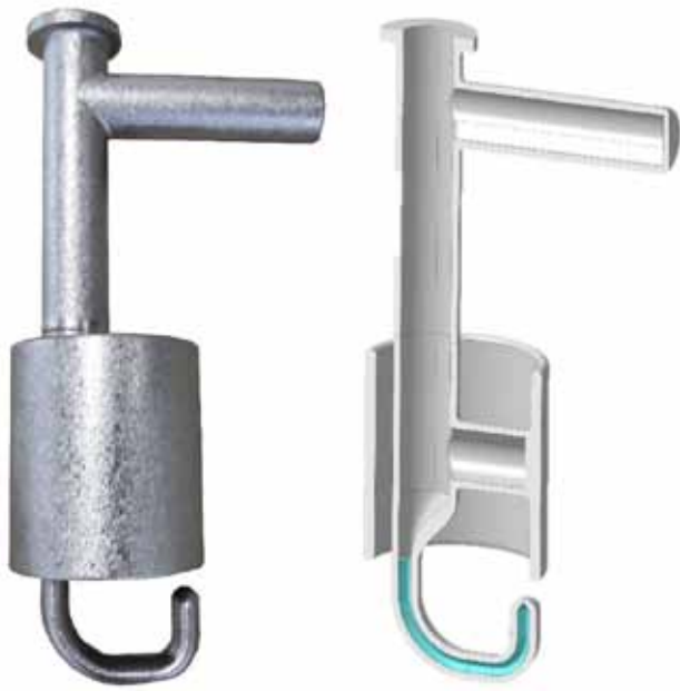
(Above) This HOM coupler prototype made of niobium has cooling channels going right down to the point of the hook, where the electromagnetic fields are intense. (Image: CERN)
