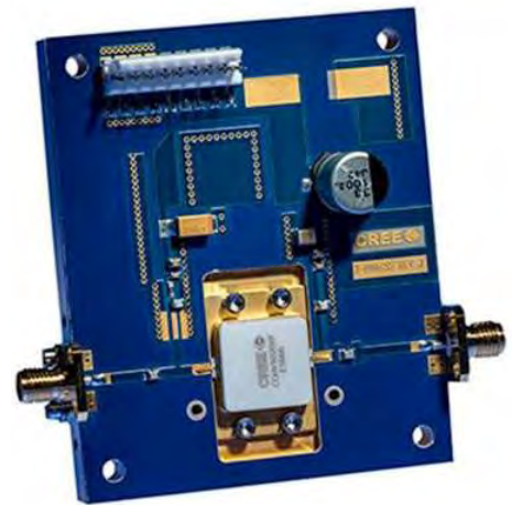
An example of a RF GaN power amplifier (Photo: Cree)
