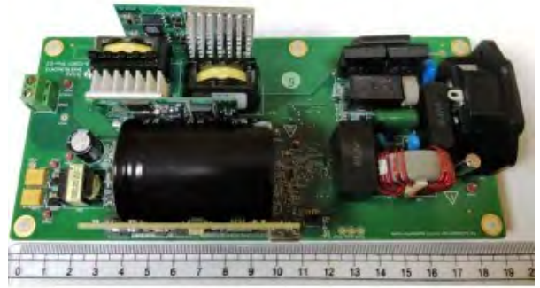
A TIDA 00961 GaN board by Texas Instruments, designed for telecom, servers and industrial power supplies refers to tantalum capacitors (photo: Texas Instruments)
