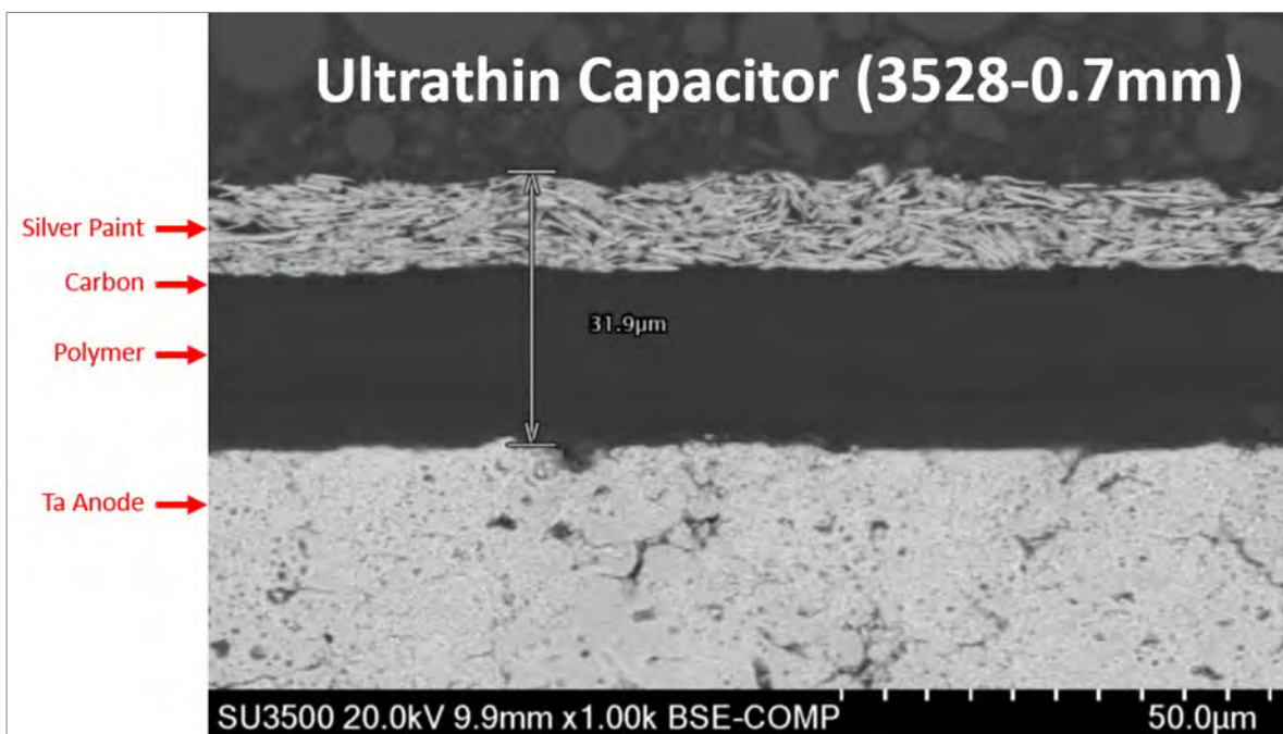
Figure 12: Ultra-Low Profile Capacitor cathode layers
