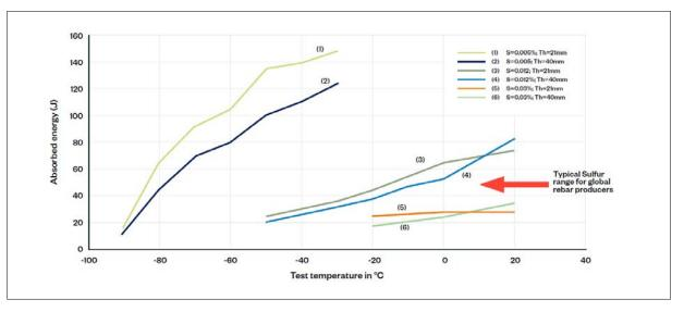
Figure 2. Sulphur effect on Charpy V toughness in transverse direction Grade 50 plate [4]
