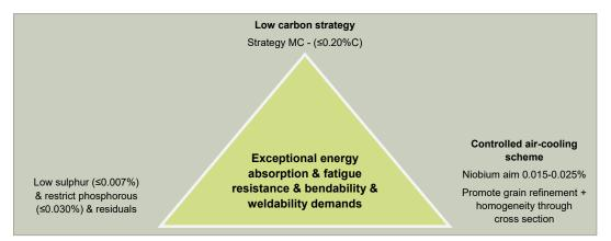
Figure 4: Next generation reinforcing bar process/product metallurgy priorities
