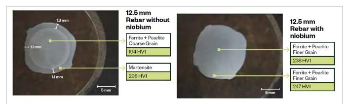
Figure 3. Water-cooled and air-cooled rebar comparison [7]
