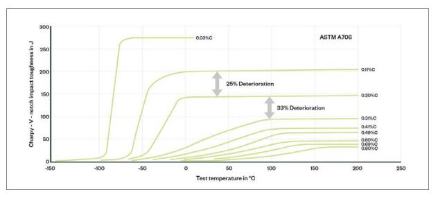
Figure 1. Impact toughness at temperature for various carbon grades [3]
